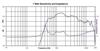
Figure 17: Frequency response and impedance at 1w/1m
