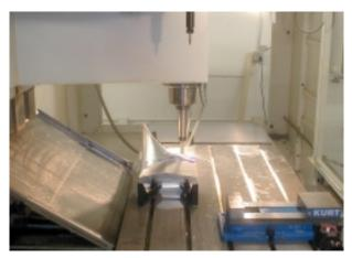
Figure 9: CNC machining-center fabricating a production horn tool.
