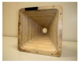
Figure 10: CNC-milled prototype of PT-F77HF waveguide.
