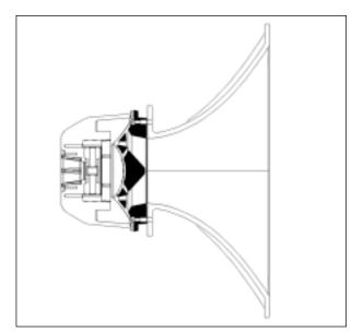
Figure 7: CMCD-81H section-view with PT waveguide.
