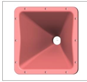
Figure 8: CAD model of PT-F77HF waveguide.
